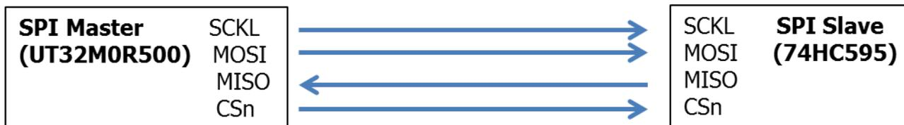
**Figure 1: SPI master/slave communication**
