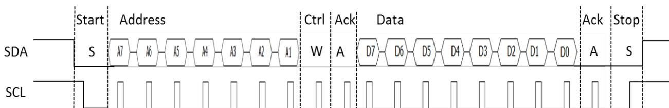
**Figure 4: Master and Slave Write Interface**
