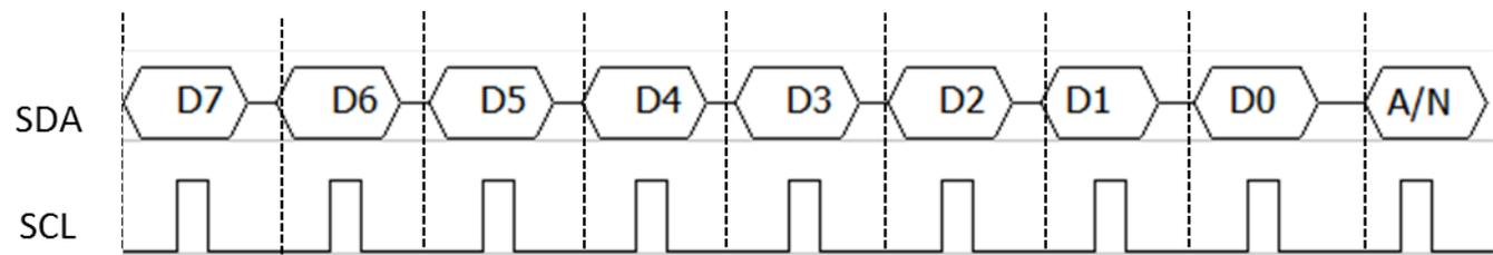
**Figure 3: I2C master/slave data transfer**
