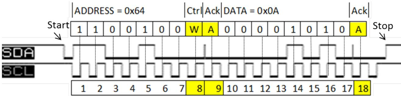
**Figure 5: I2C Write Interface Timing Diagram**
