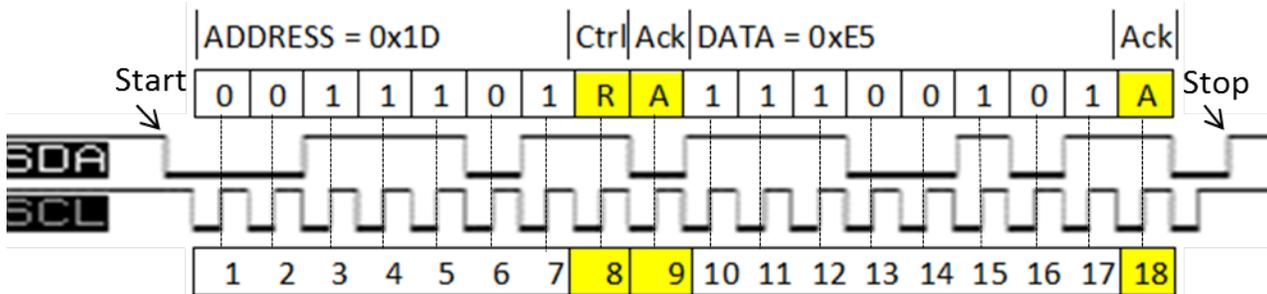
**Figure 7: I2C Read Interface Timing Diagram**
