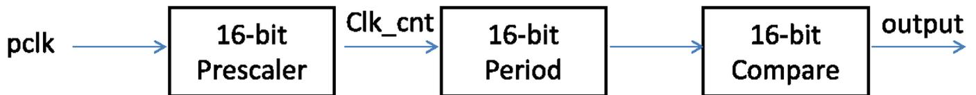
**Figure 1: PWM basic diagram**
