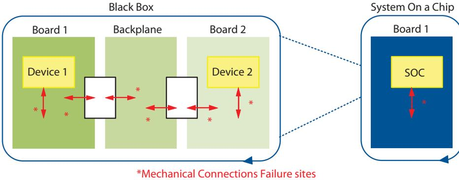
**Figure 3: Mechanical Failure Site Comparison**
